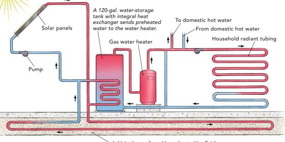
A 16-in. layer of sand is preheated by fluid coming directly from solar panels.
